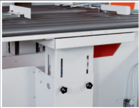
SETTING OF THE CONVEYOR HEIGHT Our R-LOCK system enables a quick change of the working height and ensures a perfect flatness between the input and the output conveyors.
