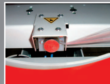
The automatic film hooking, cutting and holding unit allows the automation of the wrapping process.
